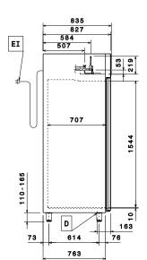
EI = Electrical inlet (power) Refrigerant Inlet = Refrigerant Outlet
